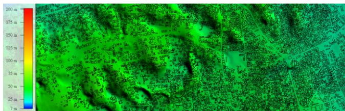
Figure2. Building Outline Overlaid on DTM
